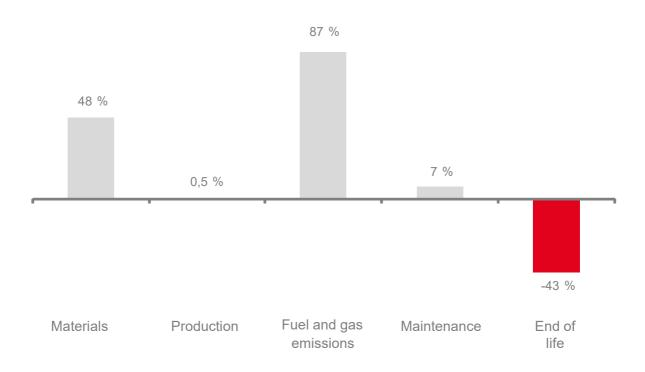
The consumption of fuel and the gas emissions resulting from it make up the greater part of the impact. The materials used for manufacturing the vehicle, particularly those introduced to meet the Euro VI standard play a significant role. This is, however, offset by their high level of recycling.
