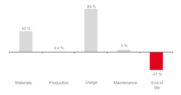
The consumption of fuel and the gas emissions resulting from it make up the greater part of the impact. The materials used for manufacturing the vehicle, particularly those introduced to meet the Euro VI standard play a significant role. This is, however, offset by their high level of recycling.
