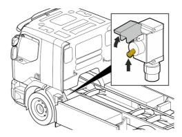
• Remove the screws (1) and remove the cover (2).
